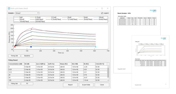
**Answer: Automatic evaluation** At the end of the experiment, iMSPR's smart analysis tool automatically performs a kinetics evaluation or steady state affinity evaluation after overlaying the sensorgrams of all the concentrations of the analytes you have run. After checking the result, you can print the result through the report button.
