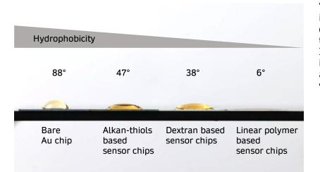
Various sensor chips made by icluebio have different degrees of hydrophobicity depending on the back-born material structure. Instead of using just one chip, improve the quality of your analysis with sensor chips of various surfaces.
