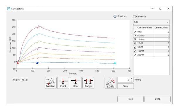
**Easy to edit for more accuracy evaluation** Now, there is no need to cumbersomely edit and analyze curves in a separate analysis tool after the experiment is over. Using the built-in iMSPR analysis tool, a curve referencing can be done with a blank concentration data, and drift correction is possible. In addition, you can easily remove outliers that may affect the results by removing spikes in the curve and using various editing functions.
